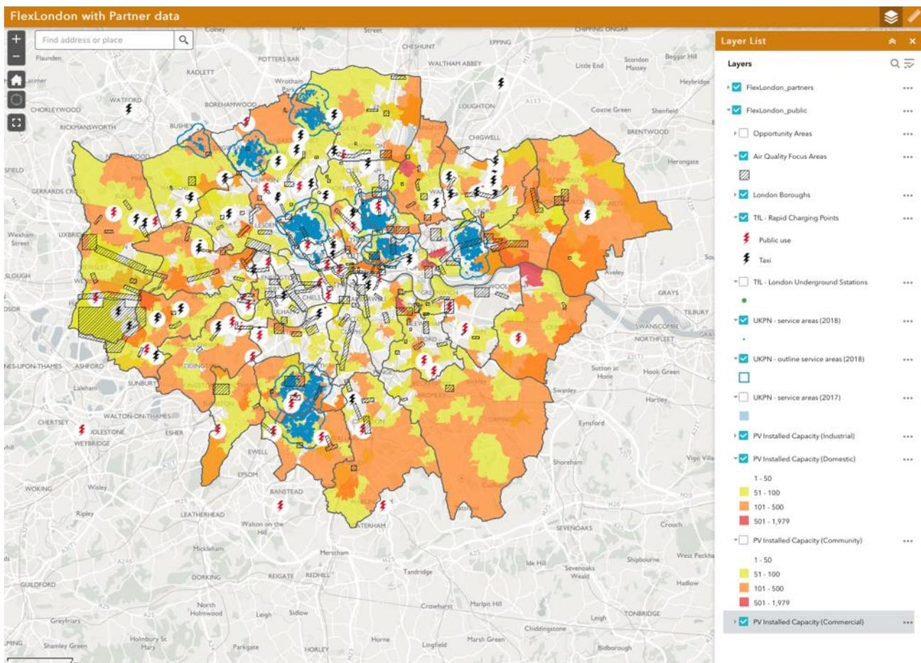
Figure 10 FlexLondon Data Visualisation, showing network constraint areas (blue), PV (orange and yellow), EV Charging (symbols) and air quality areas (grey hatched shaded areas)
